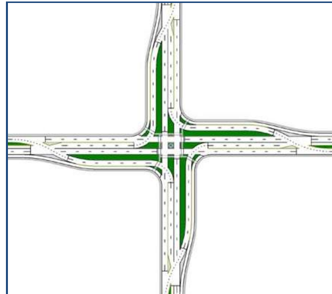
Figure 12. Continuous Flow Intersection Source (FHWA)
